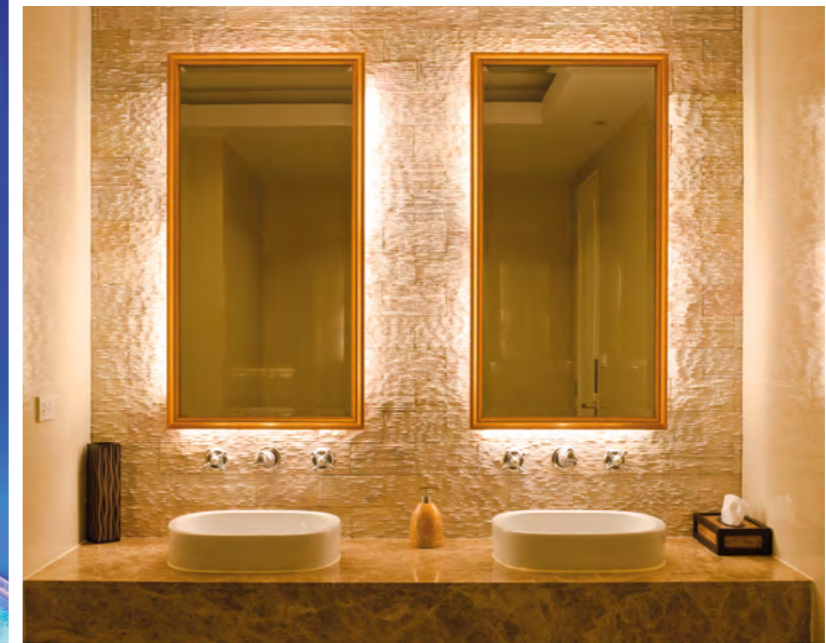
Figure 18 Use accent lighting to add flexibility, such as the use of table luminaires for reading or spotlights to highlight special items and create visual interest and stimulation. During the night, accent lighting can be used to provide lower level indirect illumination that enables navigation but is not enough to disturb.
