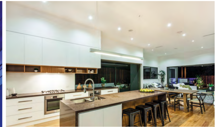
Figure 17 Use general lighting to facilitate visual acuity by effectively illuminating surfaces such as table tops, kitchen counters and desks to enable the performance of tasks, as well as floors to aid navigation.
