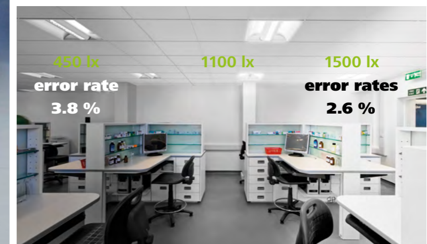
Figure 13 The impact of different illumination levels on prescription dispensing errors
